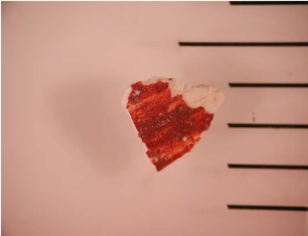
Photo 1 Sample 2 contained ground and thin red paint layer (The scale on the ruler is millimeters)
