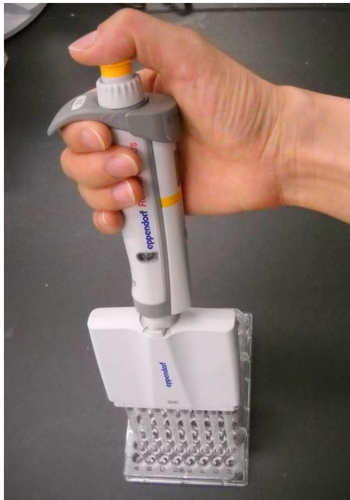
Photo 2b. Sample eluent and bicarbonate buffer were added to each well in 96-well polystyrene ELISA plate with a multi-channel pipette.
